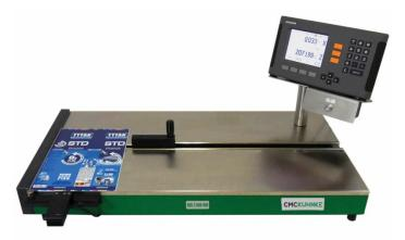
Ensure accurate slitter setups with the high-precision body blank gauge 2hdh for can making. With the help of a linear slide and heidenhain sensor combination, and another heidenhain sensor for the angle measurement, this high-precision digital gauge achieves a constant measuring force allowing for accurate, repeatable, and user-independent blank height, blank width and body blank squareness measurements.
