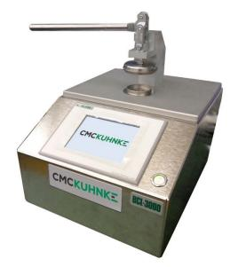
The BCL-3000L Series measures the pressure at which loose beverage ends buckle.
