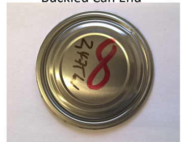
Buckled Can End
