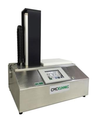
Canmakers are able to measure their beads properly and control the performance of the cans in terms of axial load and panelling strength.
