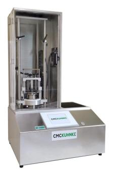
The Dome Reversal Tester is a semi-automated buckle tester designed to determine the exact pressure at which the bottom dome of a can begins to buckle.
