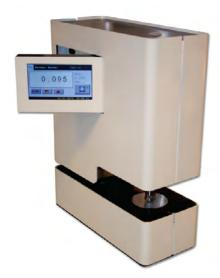
TMI Model **49-56-00-0003** is configured with a 10 mm diameter/12.5 kPa (0.393 inch/1.81 PSI) pressure foot and meets both ASTM D 6988 and ISO 4593.
