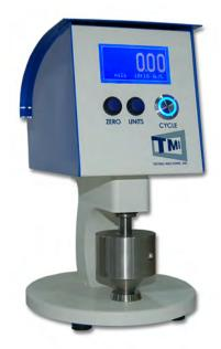
TMI Model **49-86-00-0006** is configured with a 6.35 mm diameter/31 kPa (0.25-inch diameter/4.5 PSI) pressure foot and meets ASTM D 6988 and ISO 4593.
